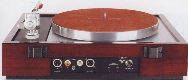
**ABOVE:** Underslung counterweight improves the stability of the TP92 arm. Thorens provides standard RCA and balanced XLR outputs plus two trim pots for 33.3/45rpm speed adjustment over a ±6% range. 3-pin DIN connects to the external PSU [below]
